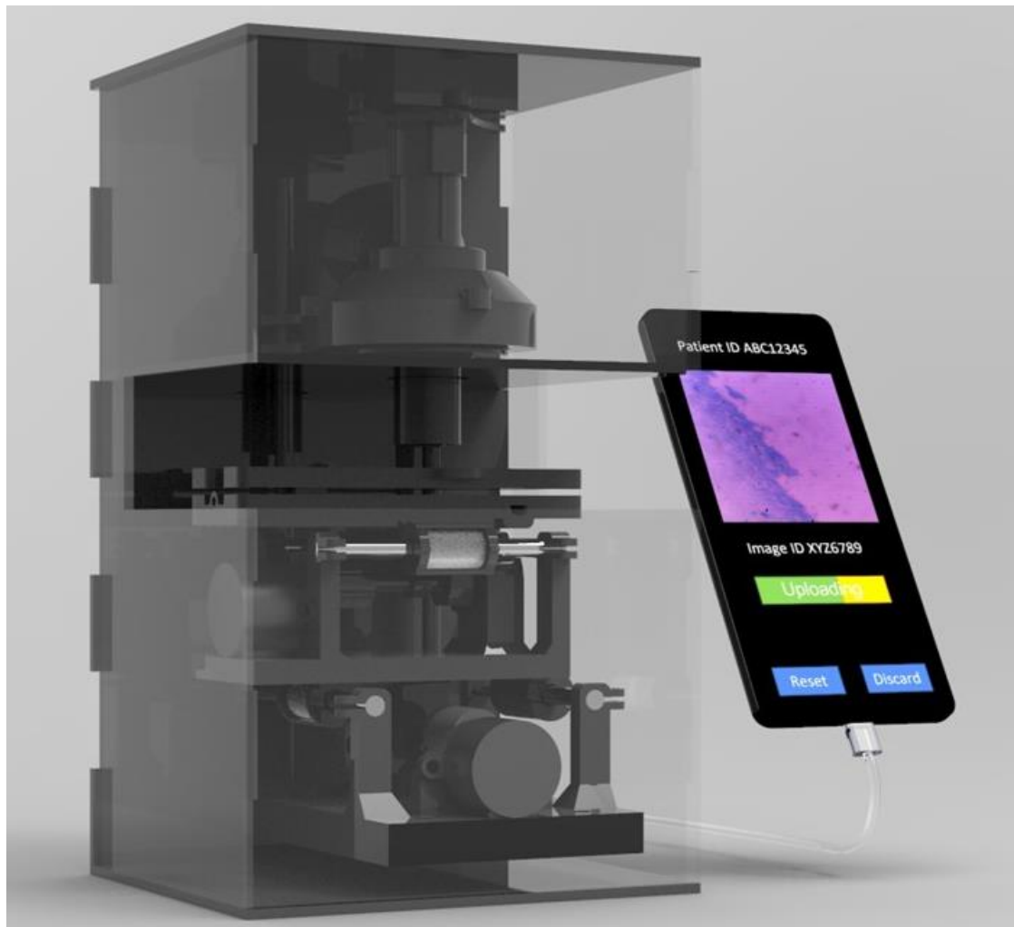
Schematic representation of a cytology scanner with a smartphone for data transfer and visualization.
