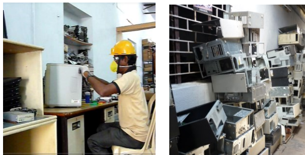
Figure 2. (i) A dismantler dismantling a CPU (left) (ii) Stock of CPU casings retrieved after dismantling in the formal sector in Bangalore, India [4]
