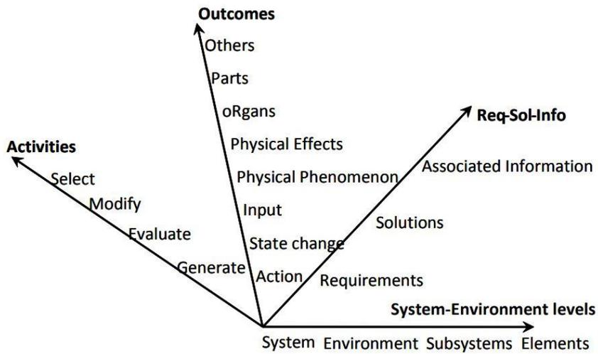
**Fig 5.** Integrated model of designing: GEMS of SAPPhIRE as Req-Sol [30]
