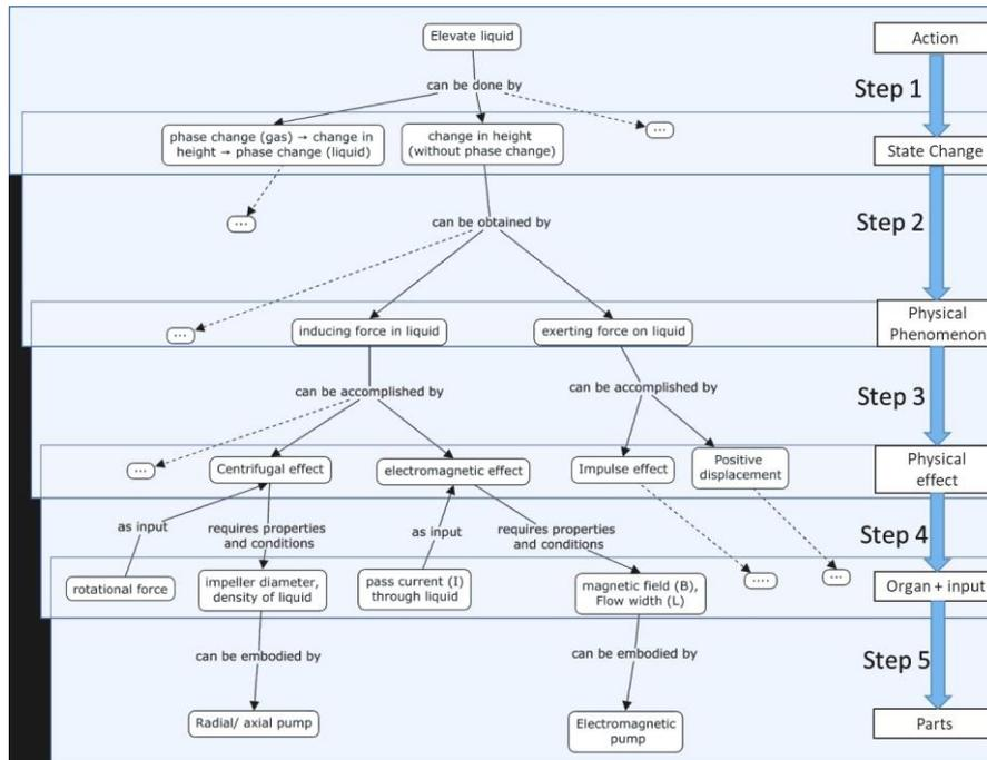
**Fig 4.** Elevating liquid illustration, reasoning with SAPPPhIRE model
