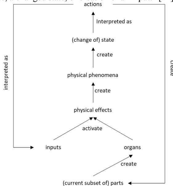
**Fig 1.** SAPPhIRE model of causality
