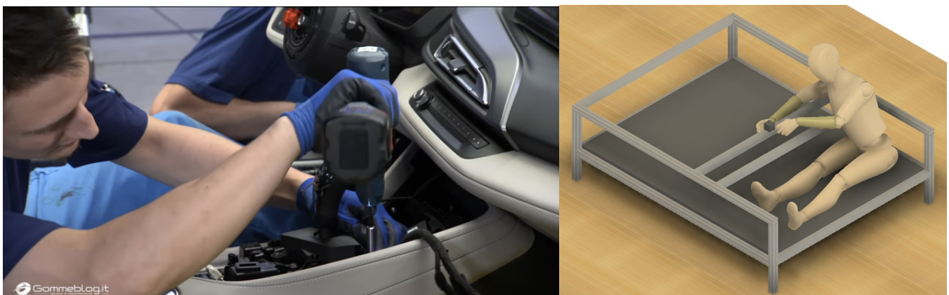
Fig.1. Task-1 on the left showing fastening of a screw on the central console of a car's dashboard [18]. CAD model of the rig for task-1 on the right.
